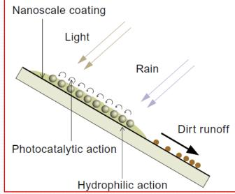
• Self-cleaning paints, textiles: Paints are relatively thick coatings in comparison to the thin coatings on self-cleaning glass. Titanium Dioxide, Zinc Oxide, and other kinds of nanoparticles are used in paints to provide the photocatalytic action.
